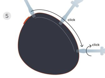
Gently slide the screwdriver along the edge of Activ5, keeping the tip inside the crevice, until you get to the spot as shown in the picture. Then stop and slightly turn until you hear a CLICK. The lid is now open and you can carefully remove it.
